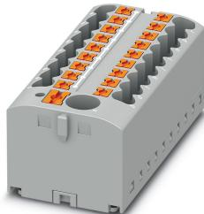
Distribution block, Basic terminal block with supply, the blocks can be bridged with one another via the conductor shaft, for corresponding plug-in bridges, see accessories, nom. voltage: 450 V, nominal current: 24 A, connection method: Push-in connection, Push-in connection, number of connections: 19, cross section: 0.14 mm<sup>2</sup> - 4 mm<sup>2</sup>, AWG: 26 - 12, width: 56.5 mm, height: 22.7 mm, color: gray, mounting type: adhesive
