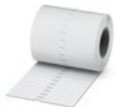
Marking foil for zack marker strip, Roll, white, unlabeled, can be labeled with: THERMOMARK ROLL 2.0, THERMOMARK ROLL, THERMOMARK ROLL X1, THERMOMARK ROLLMASTER 300/600, THERMOMARK X1.2, mounting type: adhesive, for terminal block width: 104 mm, lettering field size: 104 x 3.8 mm, Number of individual labels: 2500
